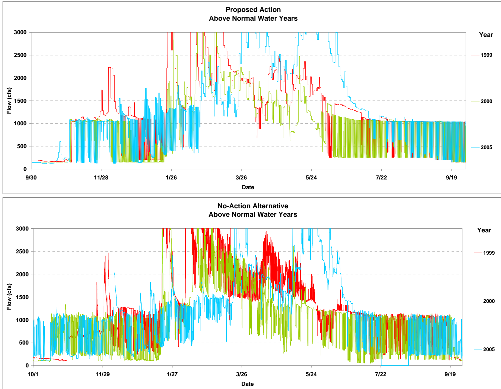
Figure 8.5-12b. Hydrographs for the Middle Fork American Peaking Reach in Above Normal Water Years under the Proposed Action and No-Action Alternative.
