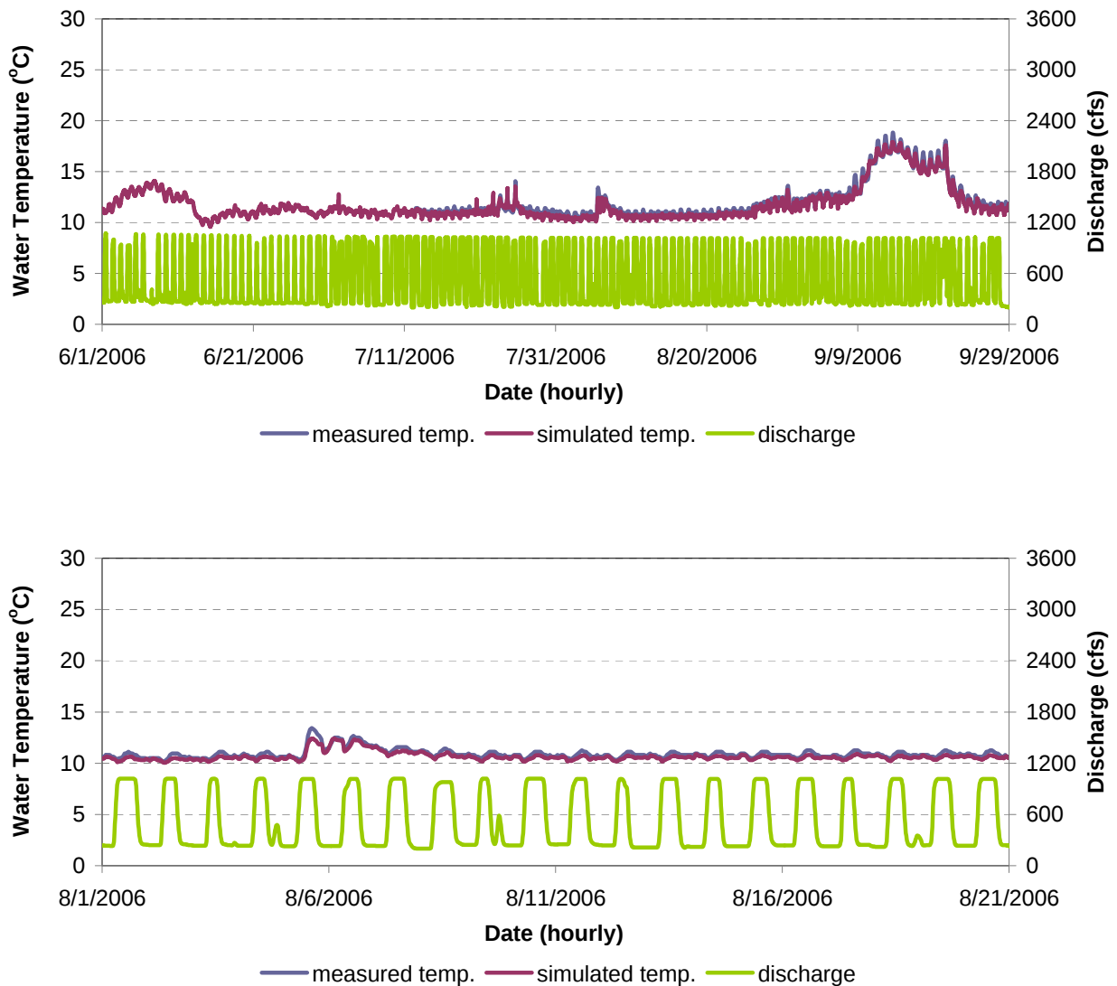
Figure F-35. Water Temperature Model Calibration Results for MF 23.1 in the Ralston Afterbay to Folsom Reservoir Reach of the Middle Fork American River for June 1 - September 30, 2006 (Top) and August 1 - August 21, 2006 (Bottom).
